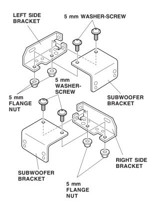
32. Remove the four screws from the subwoofer, and install the subwoofer brackets to the subwoofer with these screws.
