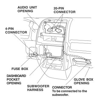
21. At the audio unit opening, connect the subwoofer harness 20-pin connector to the vehicle 20-pin connector, then secure the harnesses with one wire tie in the area shown.
