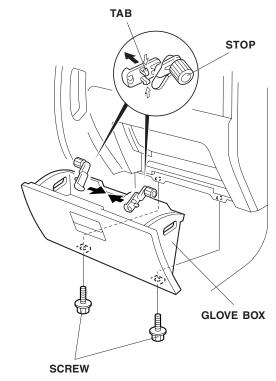
11. Remove the two screws from the bottom of the glove box, and remove the glove box.
