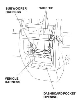
26. Route the subwoofer harness to the glove box opening, and secure it to the vehicle harness and the steering hanger beam with five wire ties in the areas shown.
