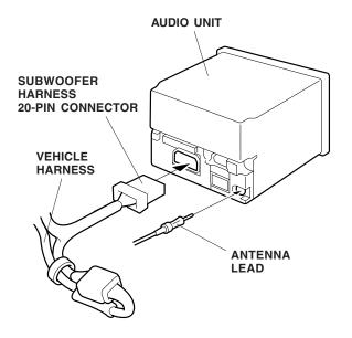
44. Slide the audio unit into the opening in the dashboard, and reinstall the four screws.
