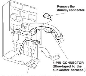
OTHER HARNESS 4-PIN CONNECTOR (Plug into the 4-pin connector bluetaped to the subwoofer harness.) 25. At the dashboard pocket opening, secure the subwoofer harness to the vehicle harness with four wire ties in the areas shown.
