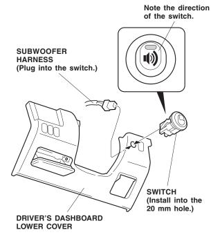
41. Plug the subwoofer harness connector into the switch.
