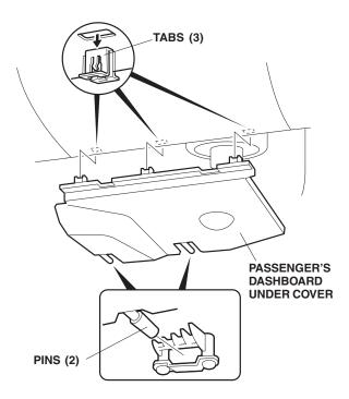
6. Open the lid. Remove the dashboard pocket (one self-tapping screw, and pull out to release the two clips and three retaining tabs).
