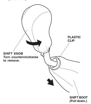
Remove the shift knob from the shift lever by turning it counterclockwise. · Remove both side covers (four tabs).
