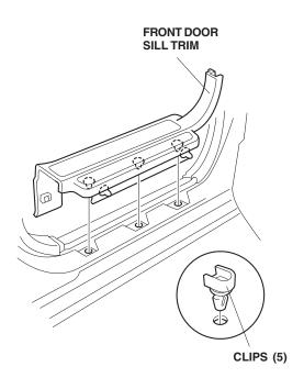
12. Reach inside the vehicle, and pull out on the bottom of the right-front door sill trim to release the two clips; then, lift the trim up to release the three clips, and remove the trim.
