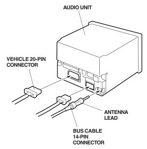
35. Slide the audio unit into the radio opening in the instrument panel, and reinstall the four screws.
