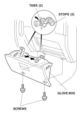
8. Remove the two screws from the bottom of the glove box, and remove the glove box.
