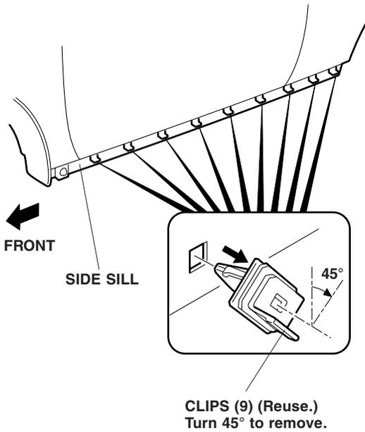
5. Slide the nine clips you just removed onto the brackets on the inside of the new left side under spoiler through the slots shown until the clips "click" into position.
