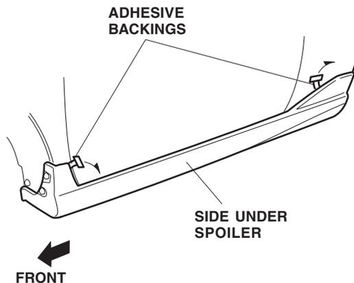
14. Turn the steering wheel all the way clockwise, and repeat steps 2 thru 13 to install the right side under spoiler.
