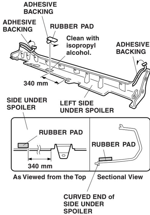
8. Attach a strip of the masking tape to the ends of the adhesive backings, and remove 40 to 50 mm from the end. Fold back the ends, and tape the ends to the front of the left side under spoiler. Note the direction of the adhesive backings.
