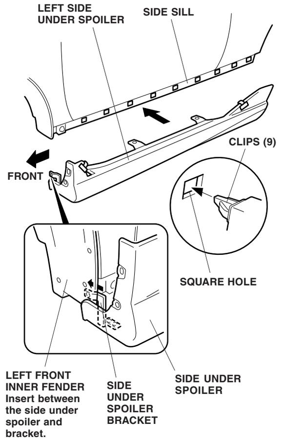
11. Install the three self-tapping screws removed in step 2 to attach the left front inner fender and the spoiler bracket.
